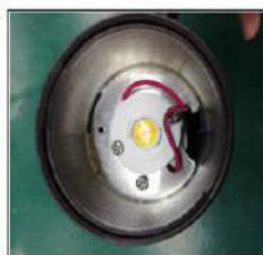
Figure3 Remove the reflector
