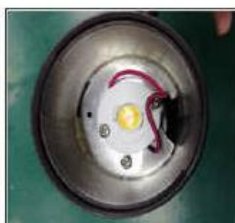
Figure3 Remove the reflector
